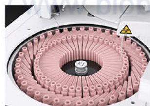
Reagent Tray 2~8°C cooling for 24 hours.
